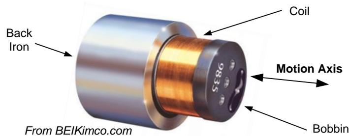
*Figure 1.6: Off the shelf Voice Coil Actuator*
