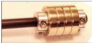
*Figure 7.15: Shaft collars constrain magnets to carbon fiber shaft*
