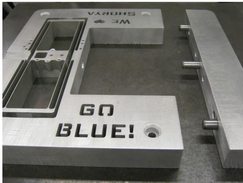
*Figure 9.10: Bearing and mover assembly (top) and removable MMA attachment plate (bottom)*
