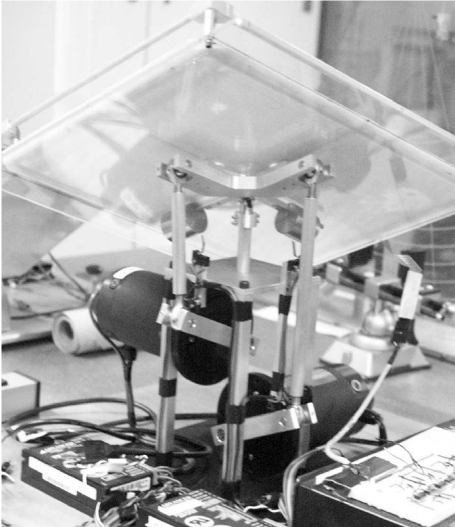
Fig. 3. The spatial linkage mechanism used for actuating the plate.
