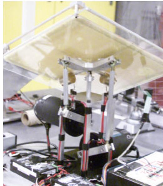
Figure 3. The spatial linkage mechanism used for actuating the plate.
