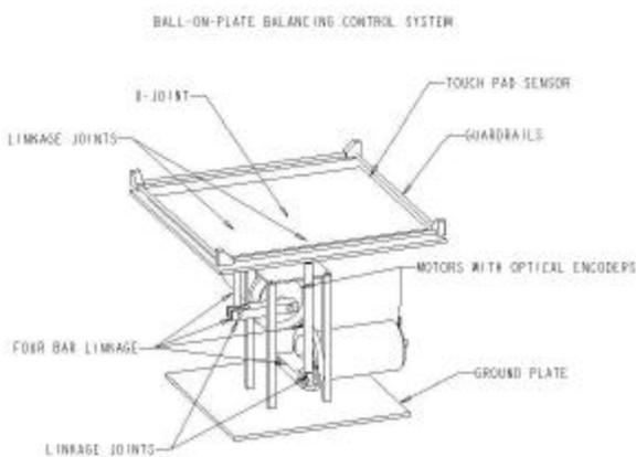
Figure 2 Ball-on-plate System Assembly
