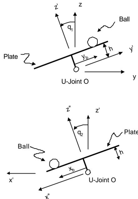
Figure 4. Physical Model of the ball-on-plate system
