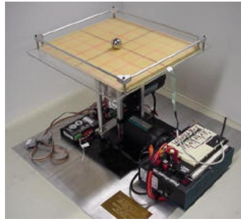
Figure 6. The ball-on-plate system in operation
