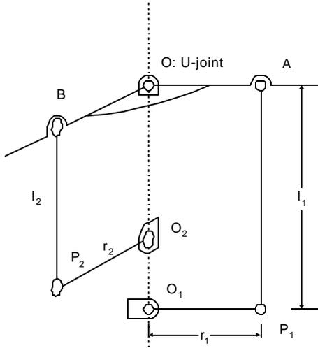
Figure 5. Plate actuation spatial linkage mechanism
