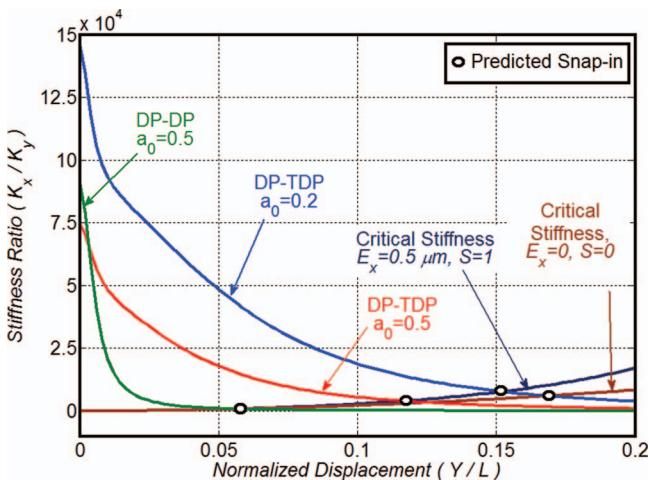
FIG. 2.  $(K_x/K_y)$  stiffness ratio for the DP-DP and DP-TDP flexures obtained via finite elements analysis. Critical  $(K_x/K_y)$  stiffness ratio curves for  $G = 5 \mu\text{m}$  and  $E_x = 0$  and  $0.5 \mu\text{m}$ .
