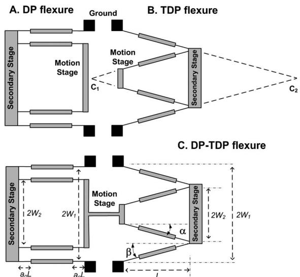
FIG. 3. Proposed DP-TDP flexure.
