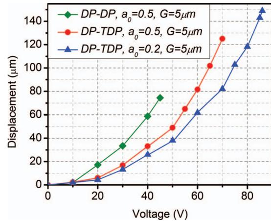
FIG. 5. Displacement measurements for comb-drive actuators based on the DP-DP and DP-TDP flexures.
