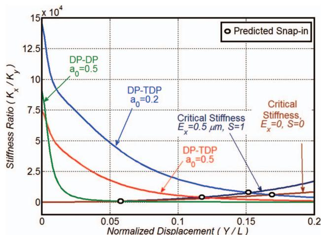
FIG. 2.  $(K_x/K_y)$  stiffness ratio for the DP-DP and DP-TDP flexures obtained via finite elements analysis. Critical  $(K_x/K_y)$  stiffness ratio curves for  $G = 5 \mu\text{m}$  and  $E_x = 0$  and  $0.5 \mu\text{m}$ .
