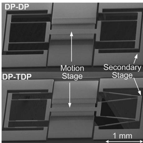
FIG. 4. SEM image of micro-fabricated comb-drive actuators based on the DP-DP and DP-TDP flexures.
