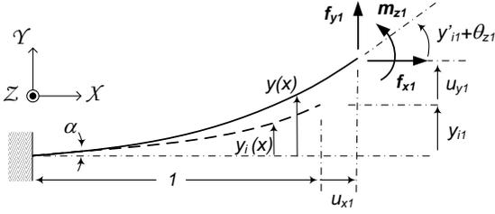
Fig. 7 Initially Slanted and Curved Beam
