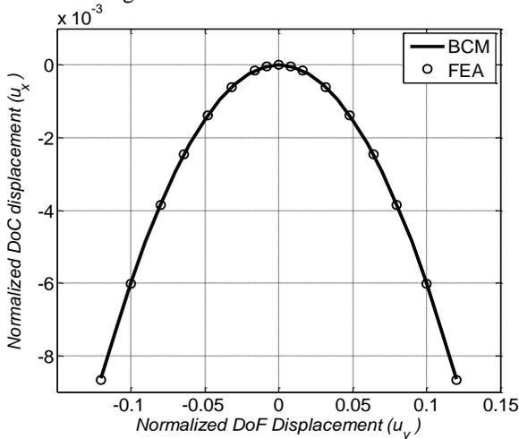
Fig.4 Parasitic axial displacement  $u_x$  (DoC) vs. transverse displacement  $u_y$  (DoF)
