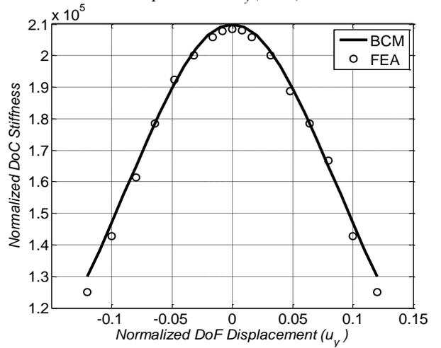
Fig.6 Axial stiffness (DoC) vs. transverse displacement  $u_y$  (DoF)
