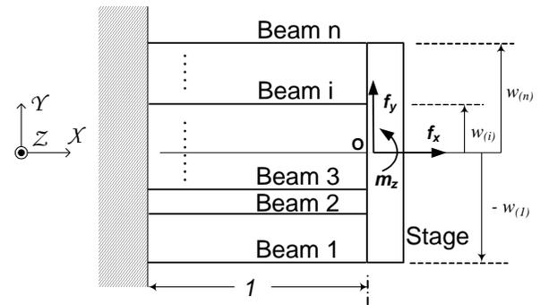
Fig.3 Multi-Beam Parallelogram Flexure
