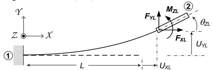
Fig. 1 Simple Beam Flexure
