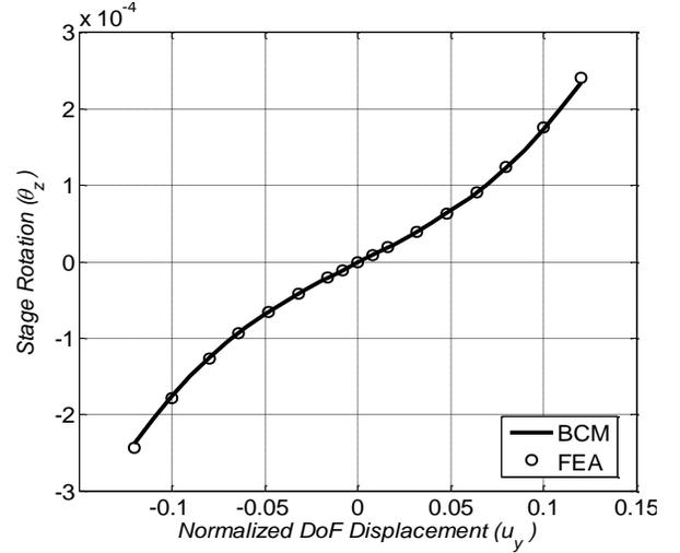
Fig.5 Parasitic stage rotation  $\theta_z$  (DoC) vs. transverse displacement  $u_y$  (DoF)
