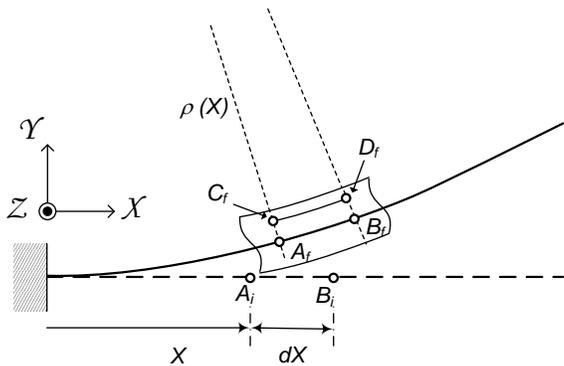
Fig.2 Undeformed and Deformed Beam Geometries
