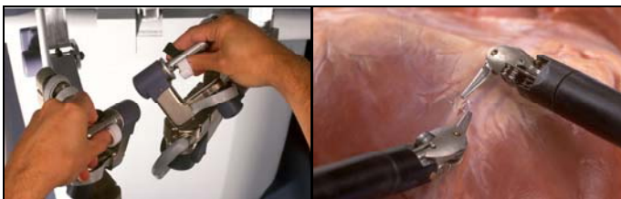
Fig. 5 Da Vinci Surgical System [27]: Input and Output
