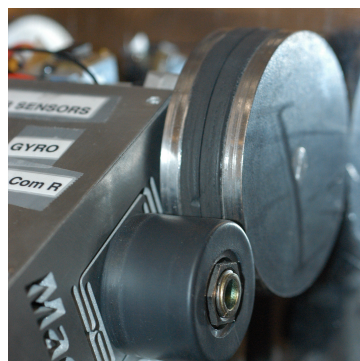
Fig. 2 Magnebot steel wheel plates and magnet core
