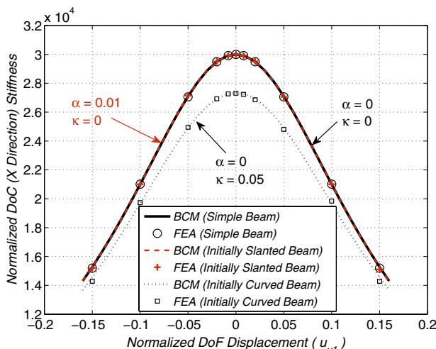
**Fig. 6 DoC stiffness versus DoF displacement ( $u_{y1}$ ) for initially slanted or curved beams**
