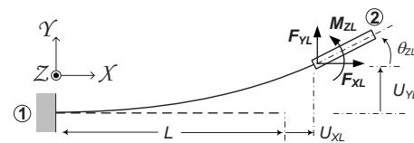
**Fig. 2 Simple beam flexure**
