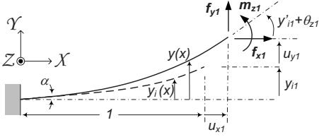
**Fig. 3 Initially slanted and curved beam**
