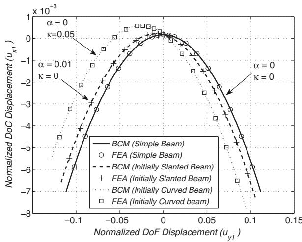
**Fig. 5 DoC displacement ( $u_{x1}$ ) versus DoF displacement ( $u_{y1}$ ) for initially slanted or curved beams**
