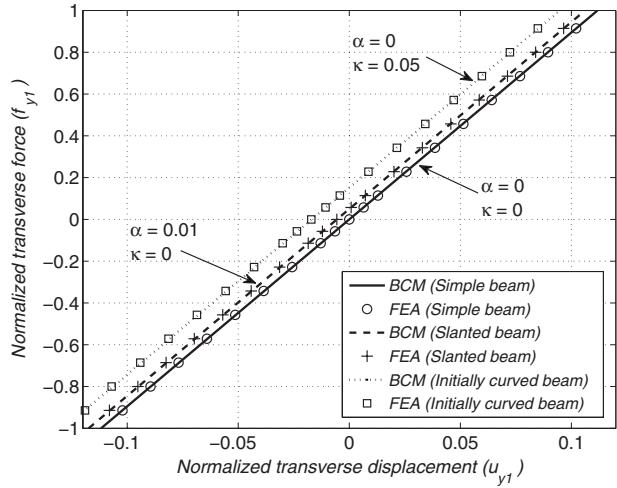
**Fig. 4 DoF force ( $f_{y1}$ ) versus DoF displacement ( $u_{y1}$ ) for initially slanted or curved beams**
