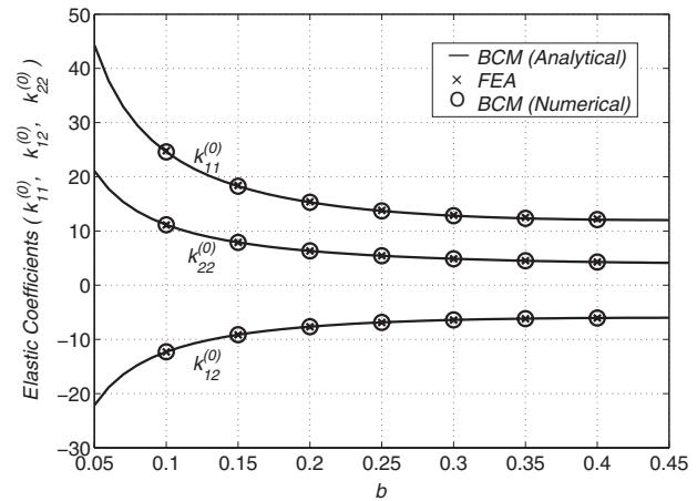
**Fig. 9 Elastic stiffness coefficients: BCM versus FEA**
