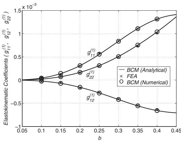
Fig. 11 Elastokinematic coefficients: BCM versus FEA
