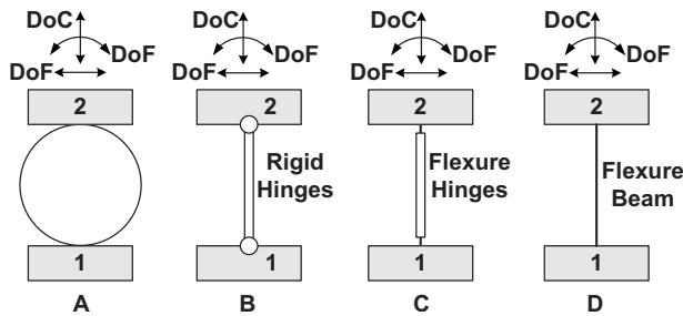
**Fig. 1 Comparison of various constraint elements**
