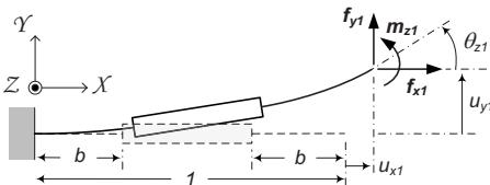
**Fig. 8 Variable cross-section beam**
