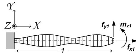
**Fig. 7 Straight beam with varying cross-section**
