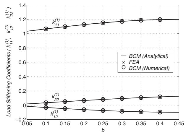
**Fig. 10 Load stiffening coefficients: BCM versus FEA**
